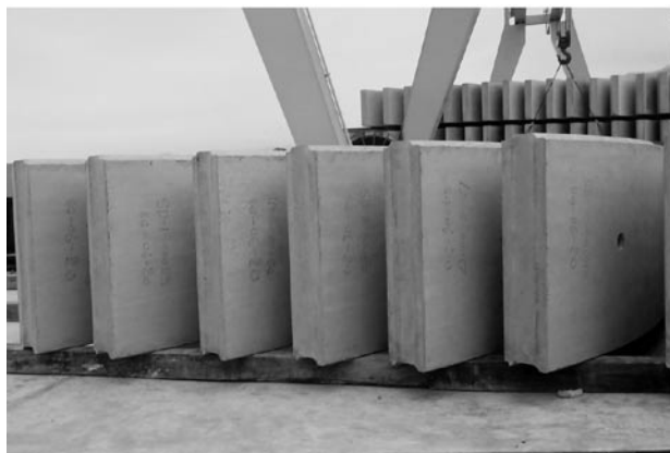
Fig. 4 The Knuckle Type Radial Joint
