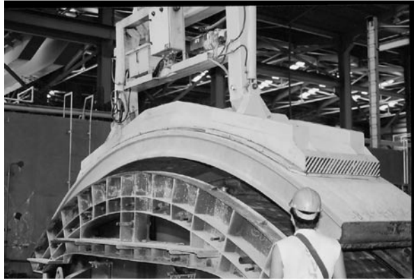
Fig. 2 The Tongue and Groove Type Circumferential Joint
